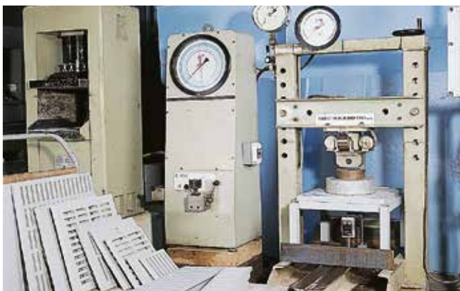
Breaking test on a light duty traffic grill.
